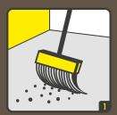
Clean the substrate of oil stains and bond inhibiting compounds. Also, remove any loose particles dirt, dust, and laitance.
